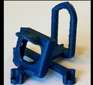
Camera/Payload mount finished part
